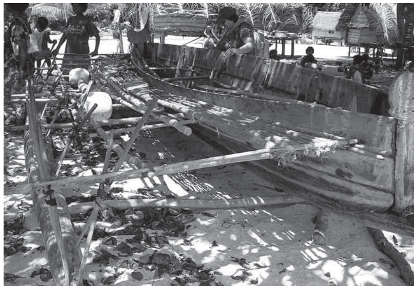
Kula canoe. Budibudi Is. Note ribs in hull. Photo: Kerry Howe
