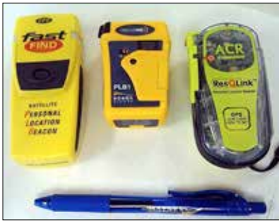
The three recommended PLB units ACR ResQLink, McMurdo Fastfind and Ocean Signals RescueMe
