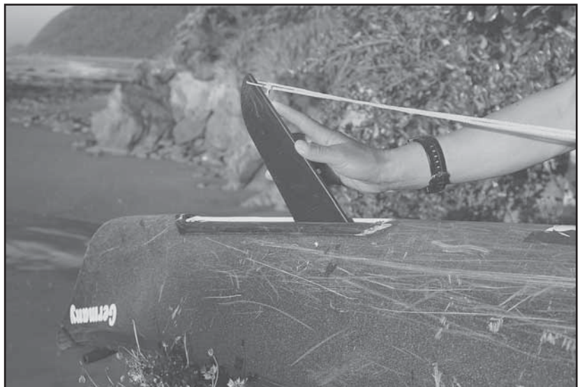
The string system Freya used to pull the skeg down after launching from a sand or gravel beach
