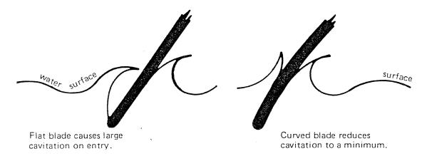
This diagram shows the difference between a flat blade and a curved blade as they enter the water. Cavitation and wave-making are greater with the flat blade.
